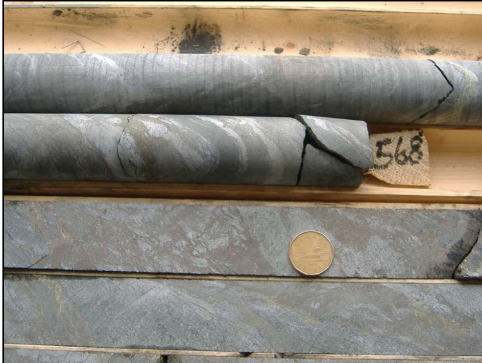
Photo 9. Drill hole "NL04-09e", 2005 Cascadia International Resources Inc. drilling. Gabbro breccia with sulphide matrix (durchbewegung texture) of pyrrhotite, pentlandite and subordinate chalcopyrite. Dollar coin is for scale (25 mm diameter).
