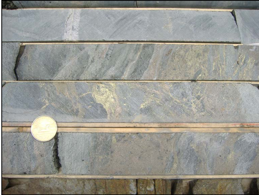
Photo 13. Drill hole "NL05-22", 2005 Cascadia International Resources Inc. drilling. Gabbro breccia with sulphide matrix (durchbewegung texture) of pyrrhotite, pentlandite and chalcopyrite. Dollar coin is for scale (25 mm diameter).
