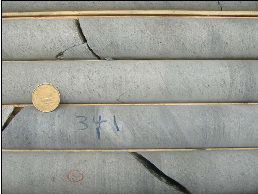
Photo 11. Drill hole “NL05-12”, 2005 Cascadia International Resources Inc. drilling. Typical massive to locally foliated host gabbro of the Norton Lake intrusion with trace sulphide. Dollar coin is for scale (25 mm diameter).
