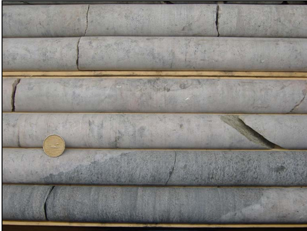
Photo 6. Drill hole "NL04-04", 2004 Cascadia International Resources Inc. drilling. Felsic dike cutting massive to foliated gabbro. Dollar coin is for scale (25 mm diameter).
