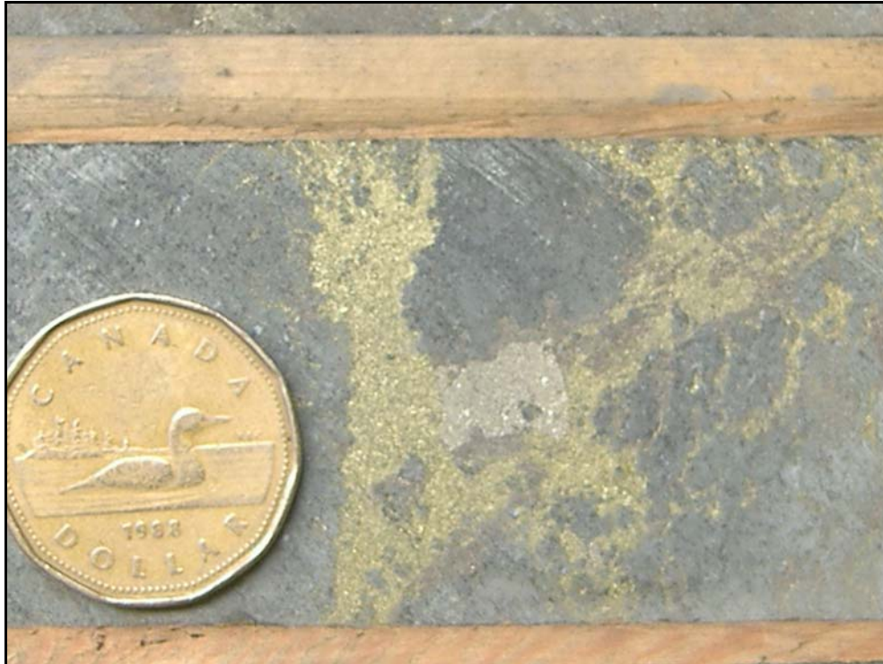
Photo 4. Drill hole "O", 2002 East West Resource Corp. drilling. Close-up of chalcopyrite vein with secondary pyrite (central area). Dollar coin is for scale (25 mm diameter).
