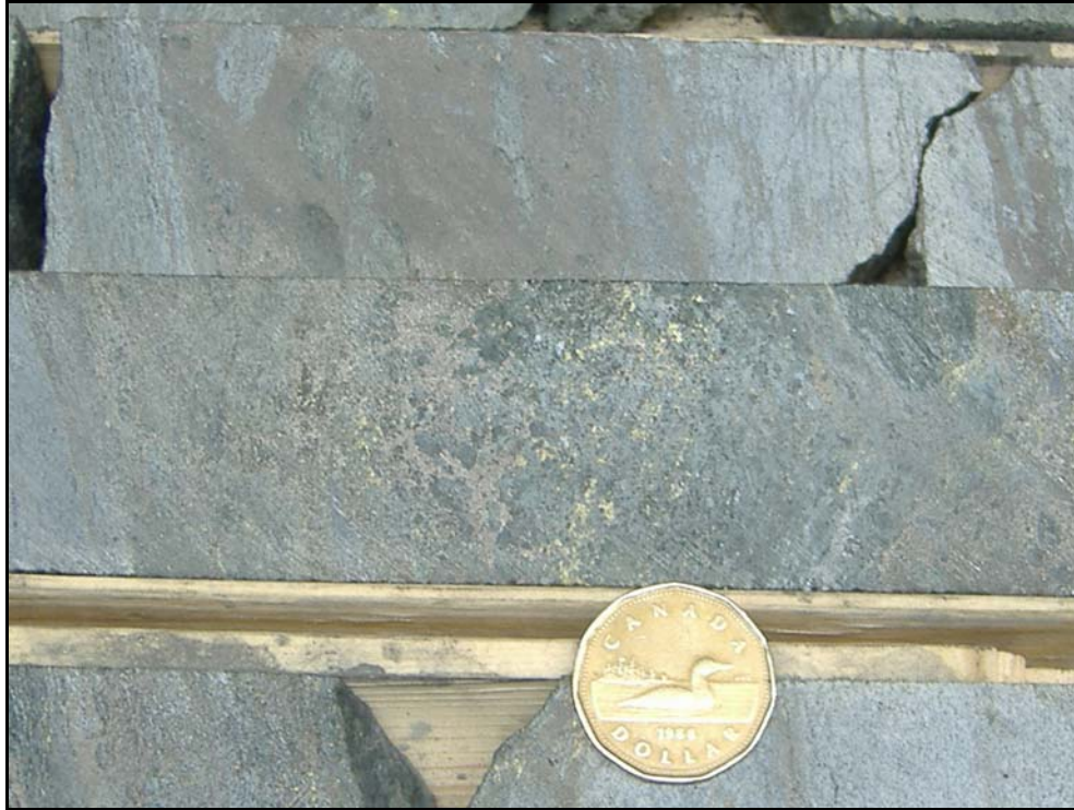
Photo 7. Drill hole "NL04-07", 2004 Cascadia International Resources Inc. drilling. Interstitial, disseminated and vein sulphide (chalcopyrite, pyrrhotite and pentlandite). Dollar coin is for scale (25 mm diameter).
