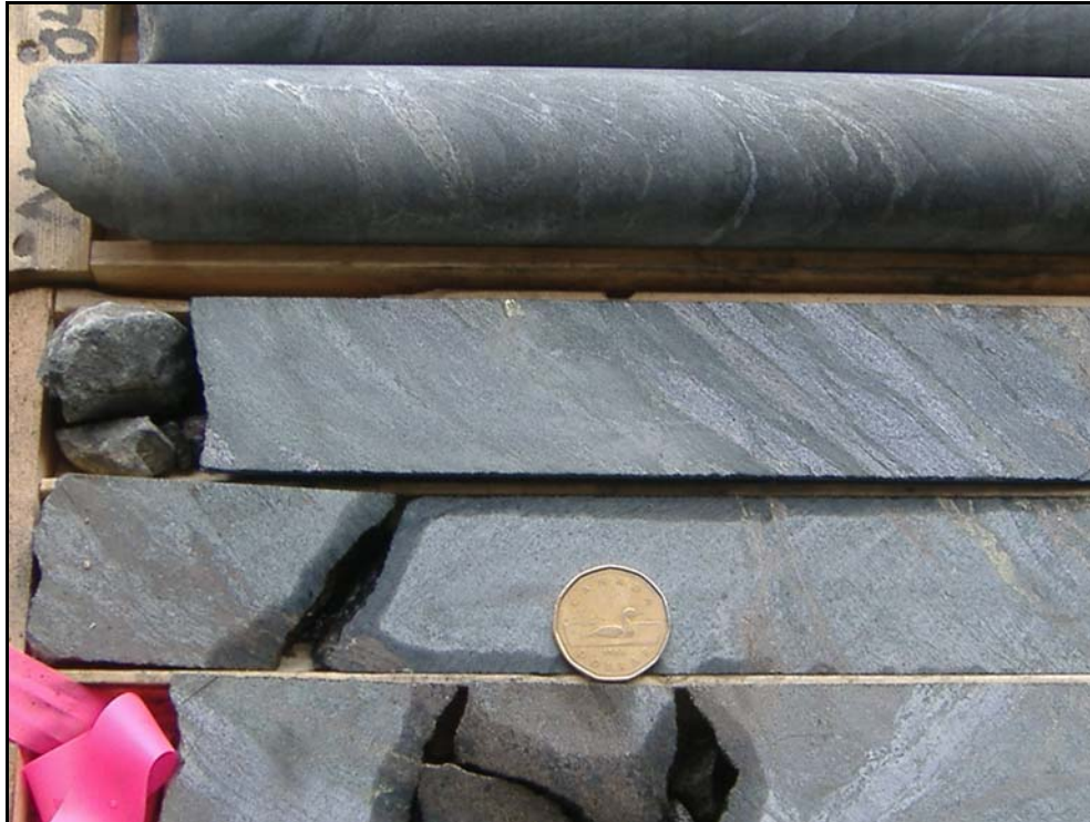
Photo 10. Drill hole "NL04-09e", 2005 Cascadia International Resources Inc. drilling. Foliated gabbro with sulphide (pyrrhotite, pentlandite, chalcopyrite) parallel and cross-cutting foliation. Dollar coin is for scale (25 mm diameter).
