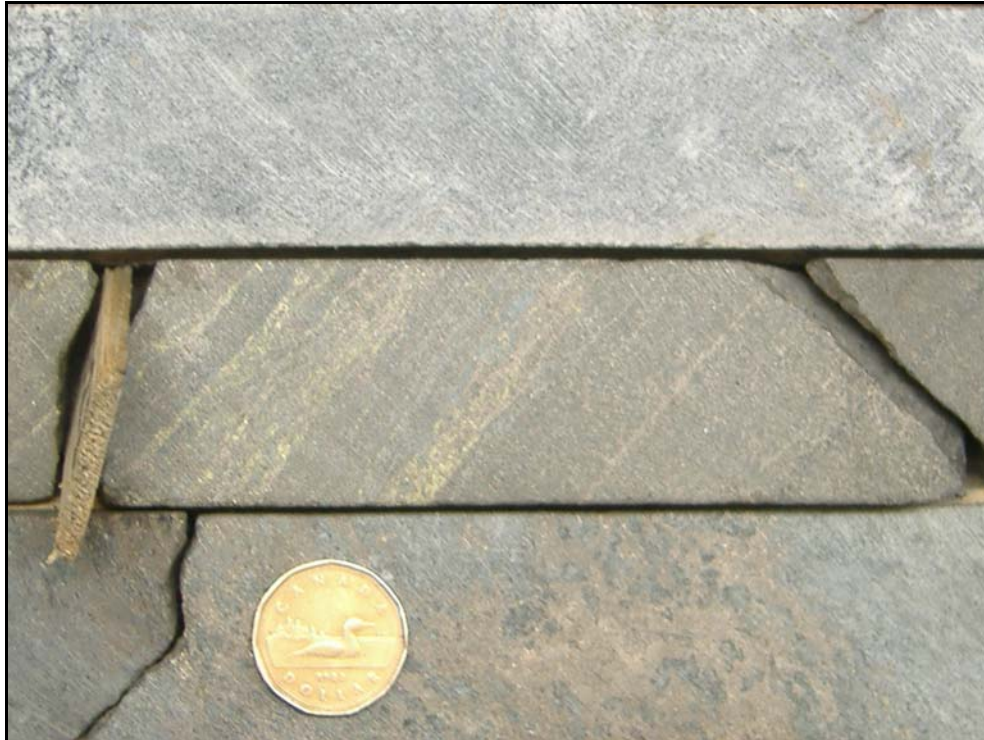
Photo 12. Drill hole “NL05-12”, 2005 Cascadia International Resources Inc. drilling. A-typical laminated massive sulphide (pyrrhotite, pentlandite, chalcopyrite) in contrast to typical massive sulphide. Dollar coin is for scale (25 mm diameter).
