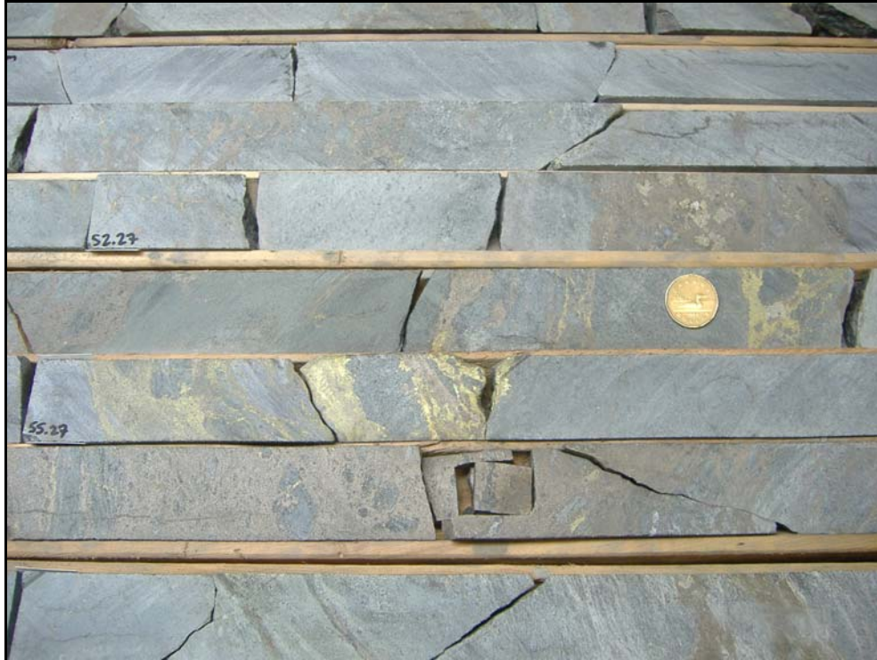
Photo 3. Drill hole "O", 2002 East West Resource Corp. drilling. Note the massive sulphide veins of chalcopyrite and pyrrhotite-pentlandite. Dollar coin is for scale (25 mm diameter).
