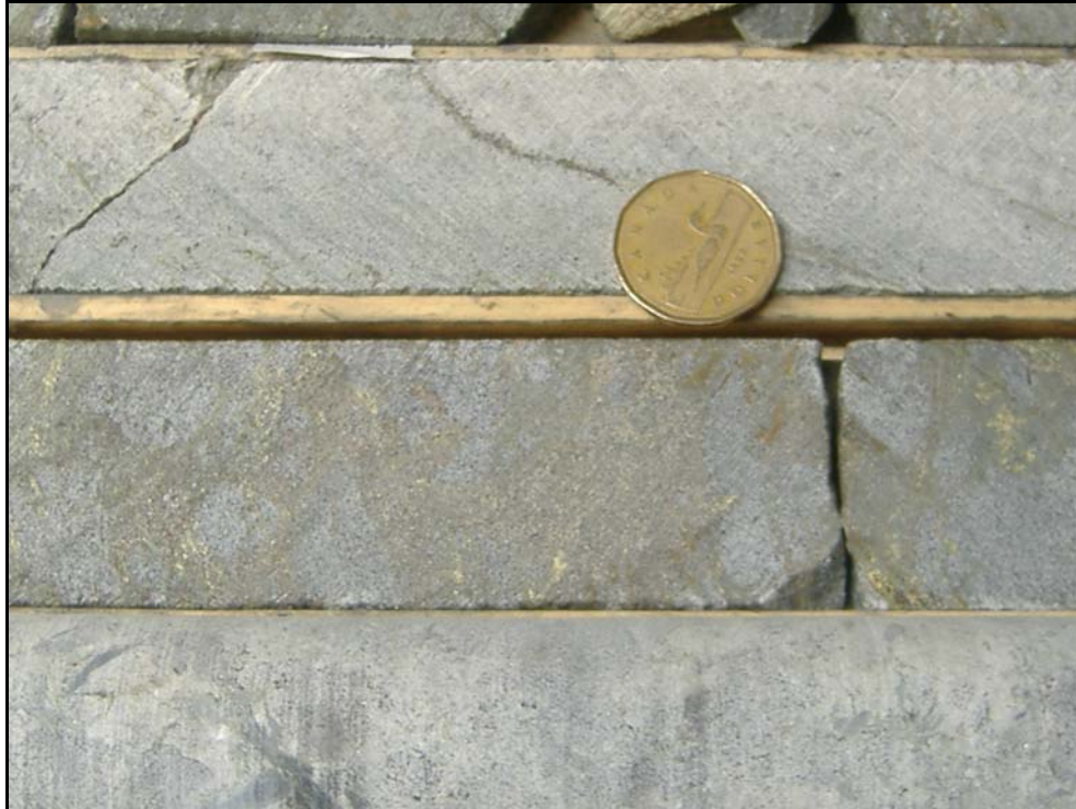
Photo 5. Drill hole "NL04-04", 2004 Cascadia International Resources Inc. drilling. Interstitial, disseminated and vein sulphide (chalcopyrite, pyrrhotite and pentlandite). Dollar coin is for scale (25 mm diameter).
