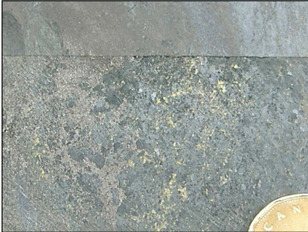
Photo 8. Drill hole "NL04-07", 2004 Cascadia International Resources Inc. drilling. Close-up of interstitial and disseminated sulphide (chalcopyrite, pyrrhotite and pentlandite). The edge of the dollar coin is for scale (about 11 mm).
